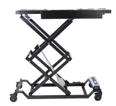
The Compact Scissor Lift Pro has been designed for where space is limited. This Lifter can take up to 35 stone and it's compact design allow it to be used in various situations. The Lifter reduces the times you need to transfer a coffin and removes the heavy lifting. The Lifter is battery powered and mains chargeable and is controlled from a mounted foot controller.
